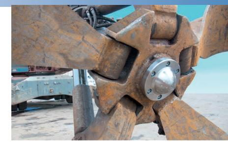
The Thermo Scientific RadEye<sup>™</sup> GR 210 brings a highly sensitive gamma radiation detector close to material being handled with a grapple. The detector is ruggedly shock mounted inside it's protective dome. This combination has proven very durable in the harsh conditions of scrap metal handling.
